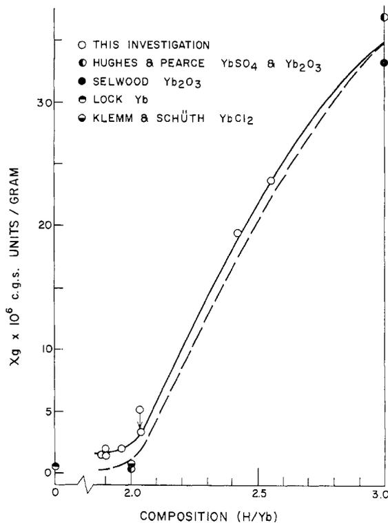
Figure 1.—Magnetic susceptibility vs. composition for the ytterbium-hydrogen system.
