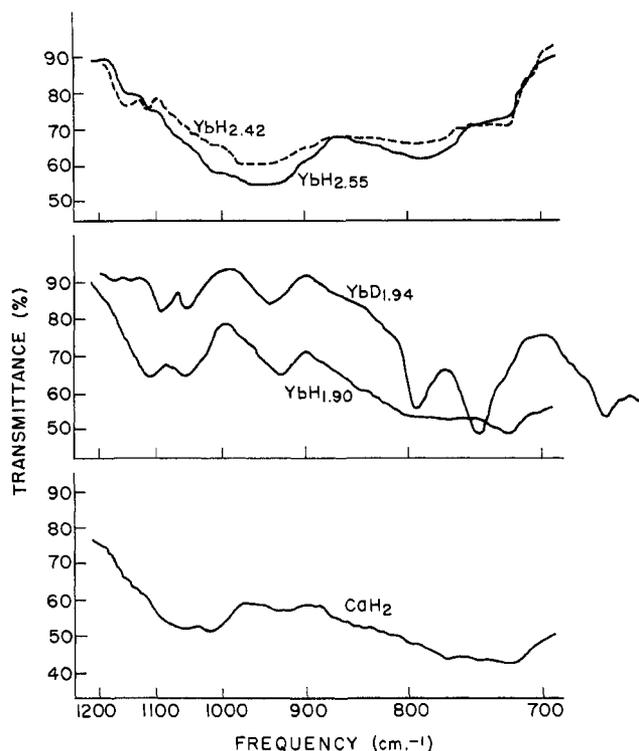
Figure 2.—Infrared spectra of  $\text{CaH}_2$  and ytterbium hydrides.
